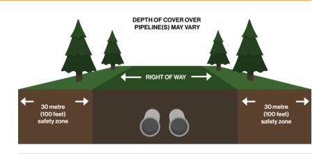
Enbridge is regulated by the NEB and must comply with specific pipeline standards and regulations. In addition to the ROW where the pipeline is located, the NEB has established a 30 metre (100 feet) safety zone on either side of the ROW to protect the pipeline, the environment and you.
