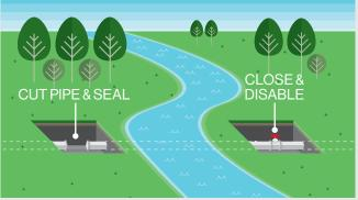
**4. Segmenting the Pipeline:** Further isolation is employed to protect water resources with the use of the permanent closure of pipeline valves or other means, including cutting and plating.
