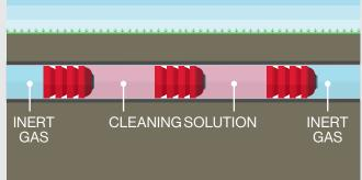
2. Clean the Pipeline: A combination of Pipeline Cleaning Tools (pigs) and cleaning solutions are used to wipe and clean the pipeline.
