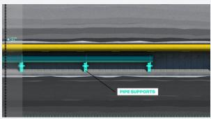
Pipe segments would be coated and welded in an onshore staging area. Supports with rollers will be bolted along the tunnel wall, and the pipe pushed along that roller system – one long segment at a time.
