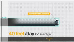
Like a giant mechanical earthworm, the tunnel boring machine would move an average of 40 feet a day, five days a week. At that rate, it's expected to take about two years to make its way across the full 4.1 miles under the Straits.
