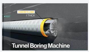
While the boring machine moves forward, it lifts segments of a 1-foot-thick reinforced concrete liner into place. Grout completes the seal.
