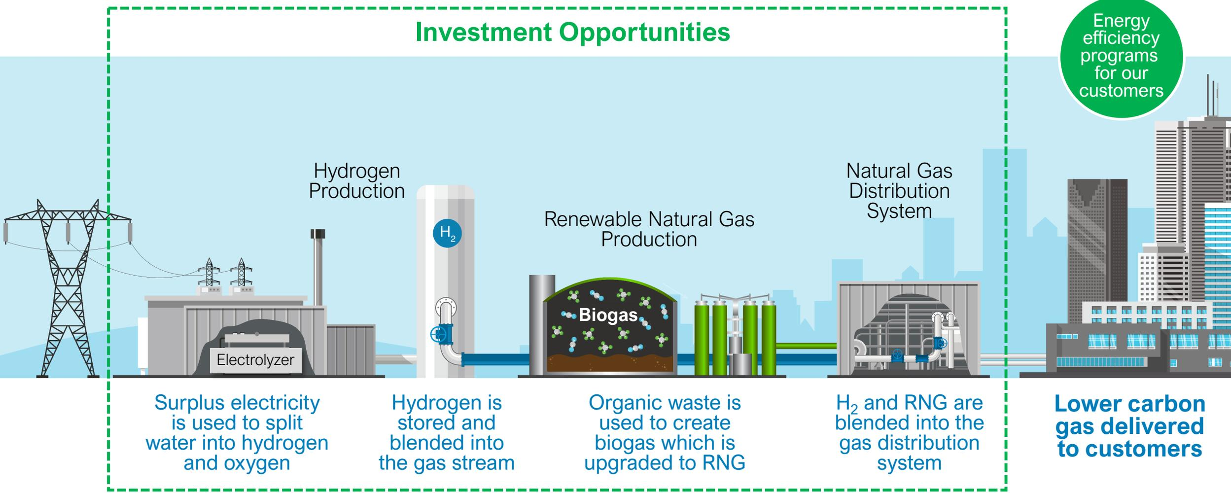
Surplus electricity is used to split water into hydrogen and oxygen
