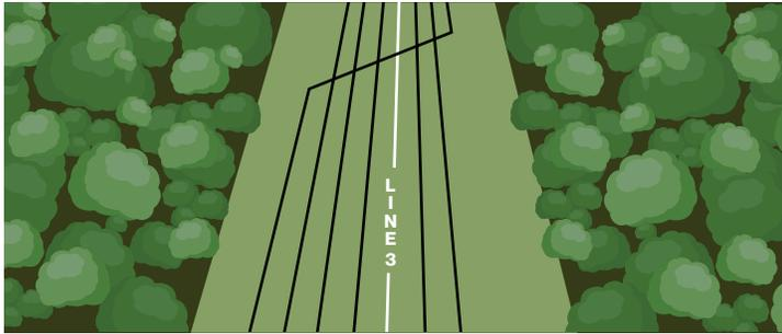
1. Following a cleaning program, Line 3, which is generally in the middle of the multiple pipeline corridor, would be located and marked. Access road locations identified.
