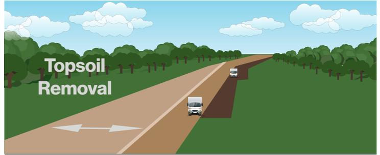
2. To protect other operating pipelines, a temporary working space would be placed and topsoil removed.
