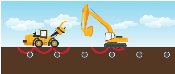
3. Timber mats are placed to protect the operating lines from the weight and stress of heavy machinery.
