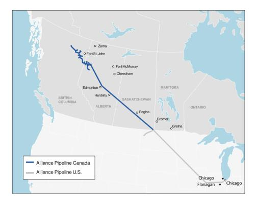
Alliance transports liquids-rich natural gas through a 3,848 kilometre underground system from northeastern British Columbia and northwestern Alberta—running through Saskatchewan, North Dakota, Minnesota, Iowa, and ending in Illinois. The Canadian portion of the pipeline consists of approximately 2,292 kilometres of infrastructure.
