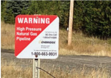
A pipeline follows a narrow, clear stretch of land, called a ROW, that allows our employees and contractors to access the pipeline for inspections, maintenance, testing, and emergencies. Approximate location of the pipeline can be determined by the pipeline marker. A few important notes when it comes to ROWs and pipeline markers:
