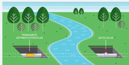
**4. Segment the Pipeline:** Permanent physical barriers are created inside the pipeline to prevent the pipeline from acting as a water conduit. This includes gate valves and permanent segmentation plugs.
