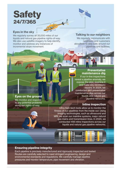
Preventative maintenance digs and in-line inspections are core aspects of our proactive inspection program which helps ensure our systems are operating safely and reliably.
