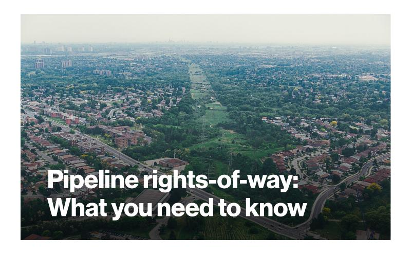
A pipeline right-of-way (ROW) is a strip of land of varying widths that may contain one or more pipelines. To deliver critically needed natural gas via our network, Enbridge must at times cross private and public lands.
