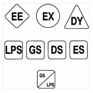
Figure 24: Markers to Identify Type of Industrial Truck
