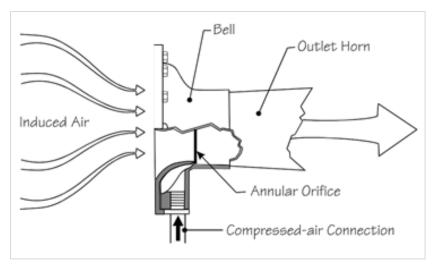
Figure 11: Air Mover Ventilator
