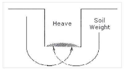
Figure 10: Heaving or Squeezing
