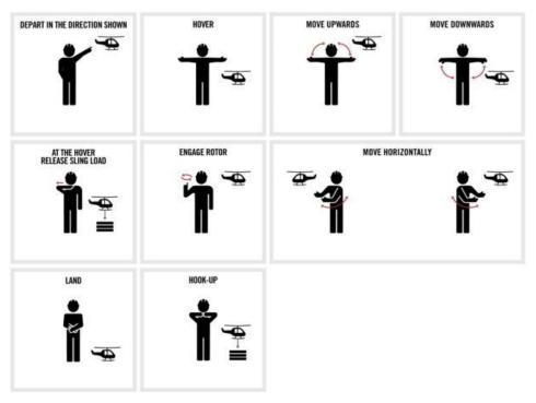
Figure 1: Helicopter Hand Signals
