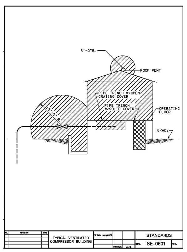
Figure 13: Typical Ventilated Compressor Building
