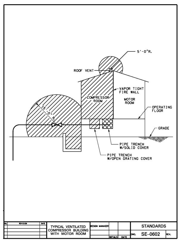
Figure 14: Typical Ventilated Compressor Building with Motor Room
