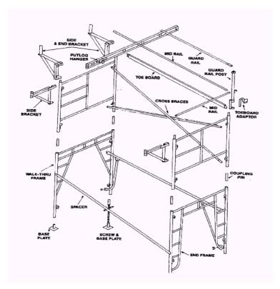
Figure 27: Tubular-Welded Frame Scaffold
