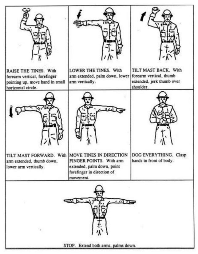
Figure 23: Standard Hand Signal for Controlling Forklift Operations
