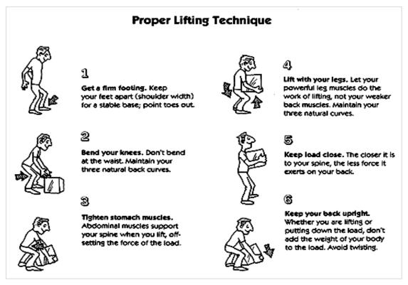
Figure 18: Proper Lifting Technique
