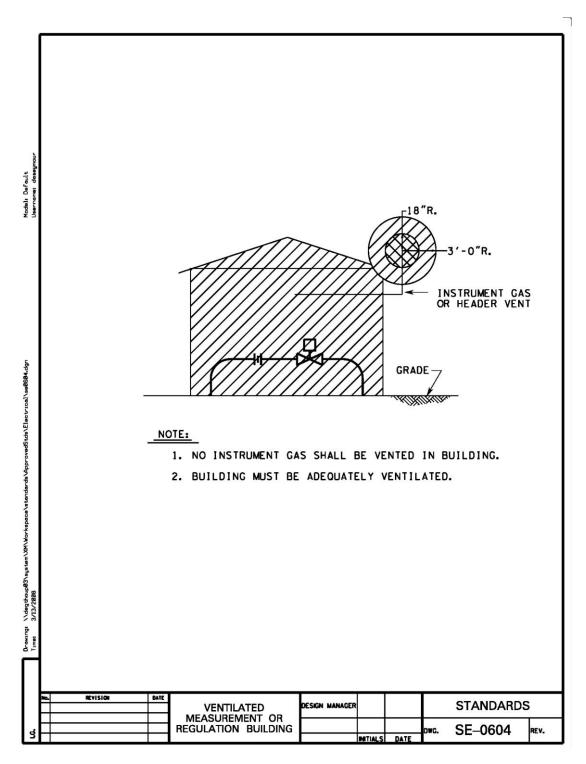
Figure 15: Ventilated Measurement or Regulation Building
