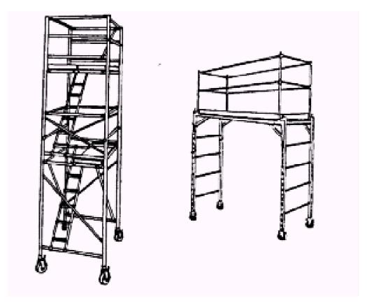
Figure 26: Manually Propelled Mobile Scaffold
