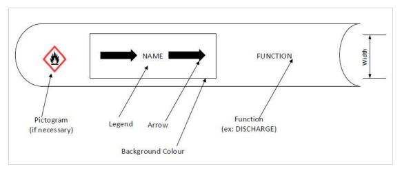
Figure 21: Example of Piping System Identification
