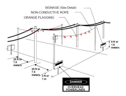
Figure 2 Crossing Overhead Power Lines
