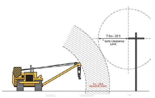
Figure 1 Example Danger Zone Between Equipment and Safe Limit of Approach Distance at known voltage of 300,000 – 350,000 Phase to Ground AC Voltage
