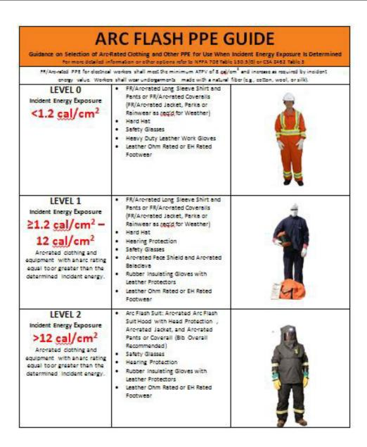
Figure 2 - Three Level PPE System
