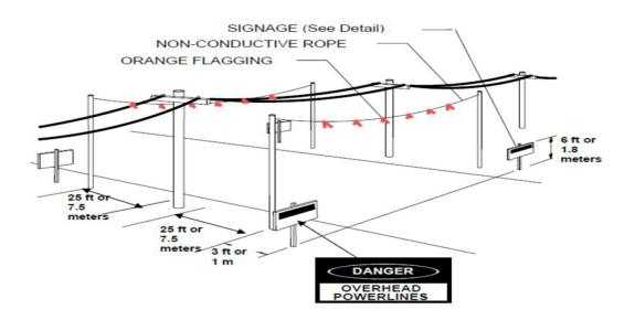
Figure 2 Crossing Overhead Power Lines
