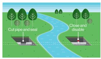
5. Segmenting the pipeline: Further isolation may be employed where necessary with the use of the permanent closure of pipeline valves or other means, including cutting and sealing.
