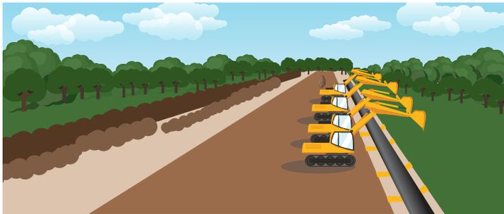
5. The pipeline would then be lifted and removed from the trench.
