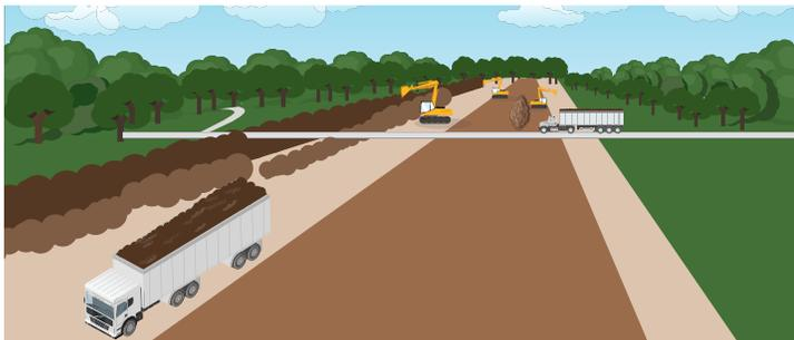
7. Trucks also haul in soil for backfill material to fill the trench.
