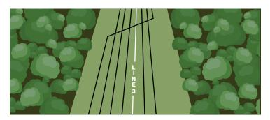
1. Following a cleaning program, Line 3, which is generally in the middle of the multiple pipeline corridor, would be located and marked. Access road locations identified.
