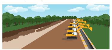
5. The pipeline would then be lifted and removed from the trench.
