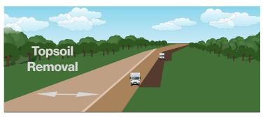
**2.** To protect other operating pipelines, a temporary working space would be placed and topsoil removed.
