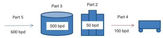
Total Capability of Refinery: 600 bpd (because Part 5 exceeds summation of Parts 2, 3 and 4)
